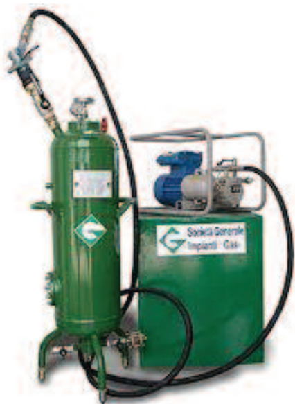
A typical bombola prover along with the ancillary pump used in Italy to verify LPG dispensers
