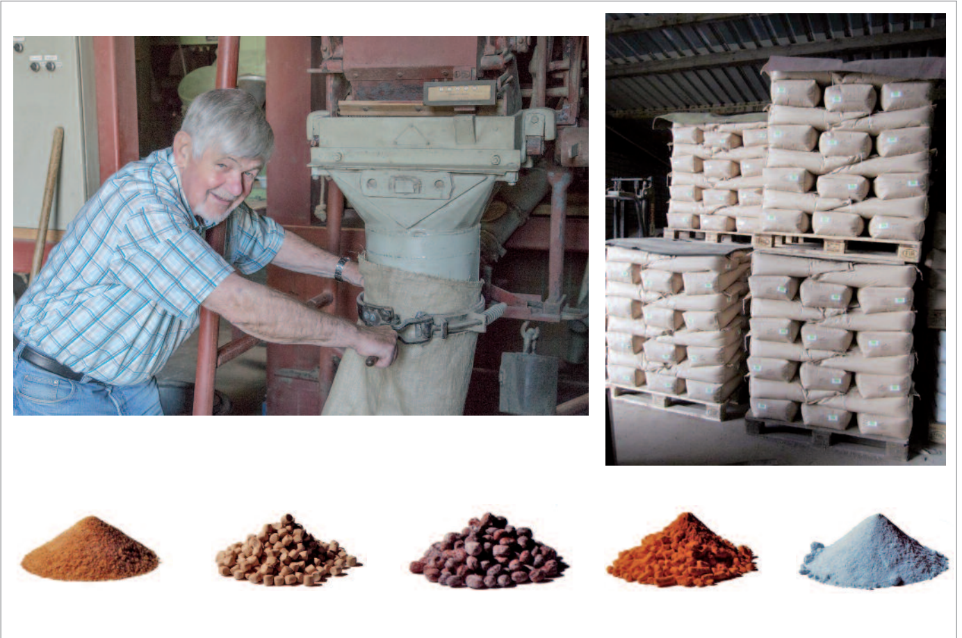
Figure 11: Left, top: Author Wolfgang Euler uses a mechanical gross weigher to bag loose products ready for delivery at manufacturer Fix-Waagen, Peter Steimel, Hennef/Sieg. Right, top: Palletizing bags. Below: Various loose products
