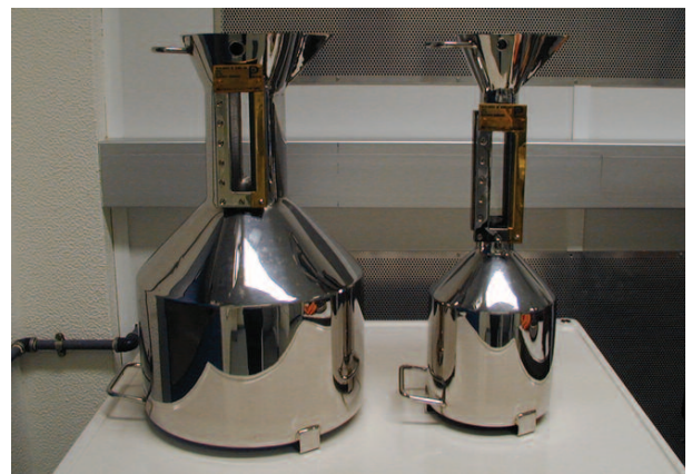
Figure 3 Stainless steel volume standard
