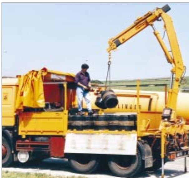
Fig. 3 Unloading two rolling weights using a remote-controlled crane
