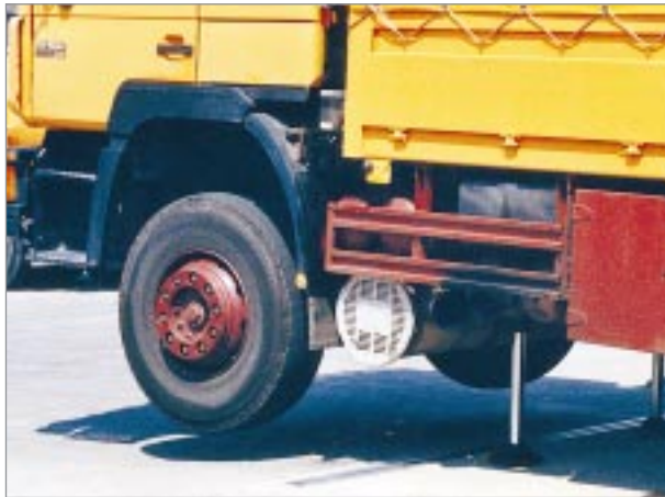
Fig. 2 Additional hydraulic support for lifting up the front axle
