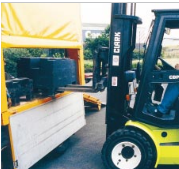
Fig. 6 Unloading a 1 t block weight
