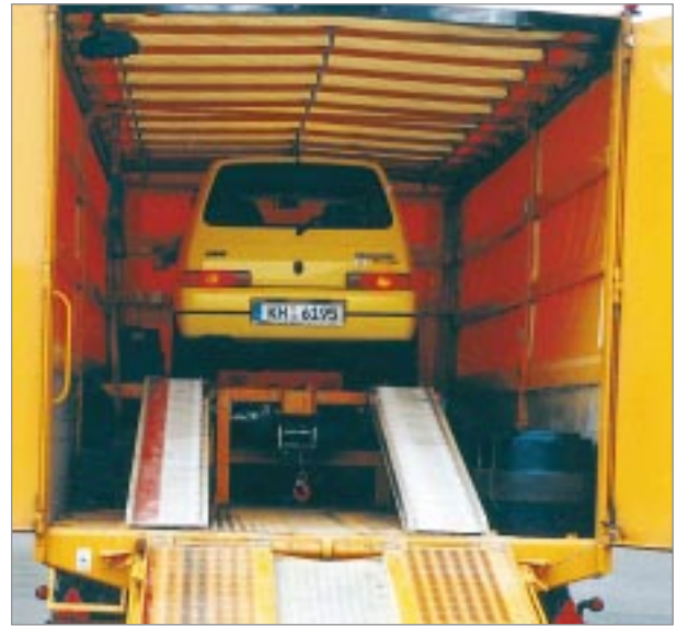
Fig. 10 Car in its final position on the trailer (beneath the car, winch for pulling up the forklift)
