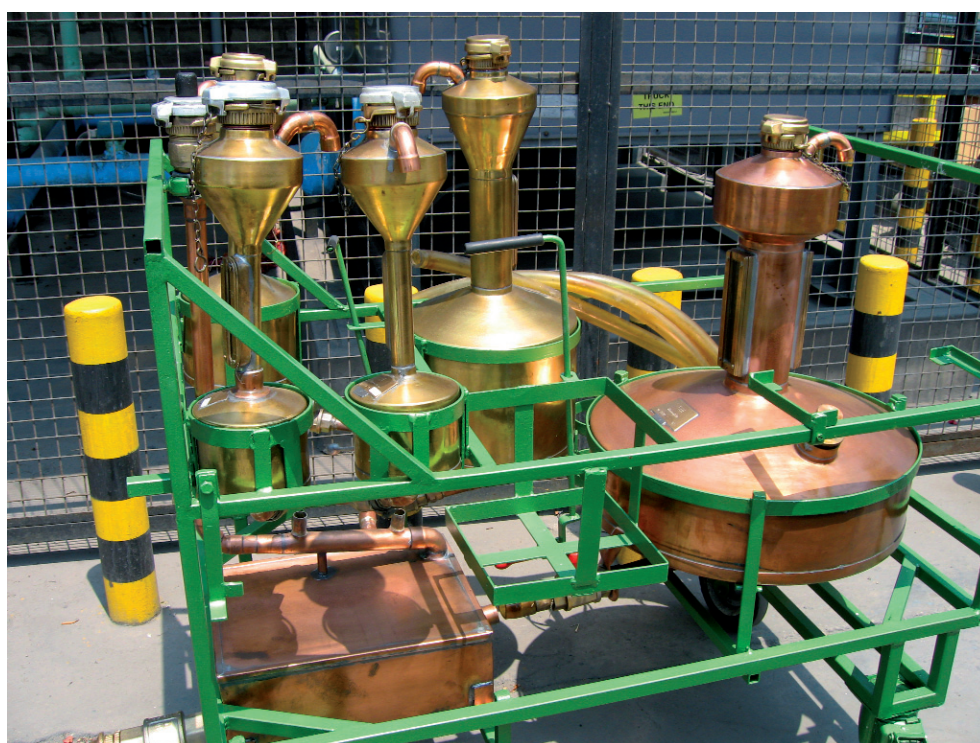
Volume standards, polished and assembled on a trolley by the receiving metrology service for the checking of petrol stations
