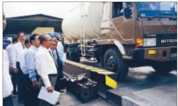
Fig. 2 Using substitution materials during the in-service inspection of a weighbridge (factory visit)
