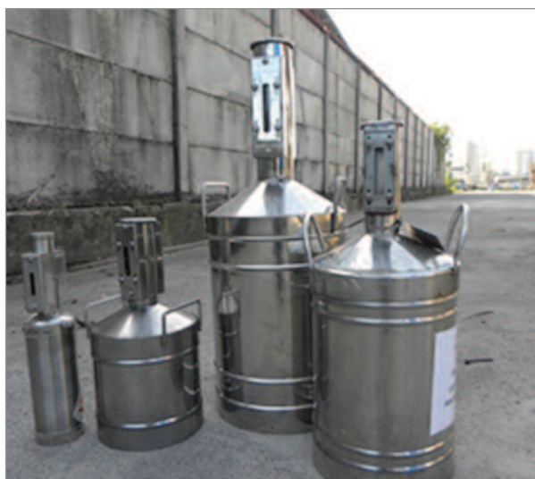
Photo 1: A set of Italian standard capacity measures for the verification of fuel dispensers (courtesy of LS Laboratorio Strumentazioni - via Padre Michele, 49 15050 Carbonara Scrivia - AL)
