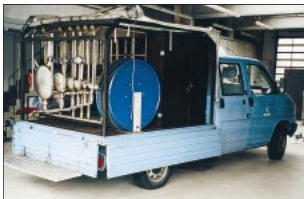
Fig. 1 Built-in testing facility in a car. While filling, the verification officer stands on the grating which is fixed to the tailboard. There is no intermediate storage of the product to be measured.
