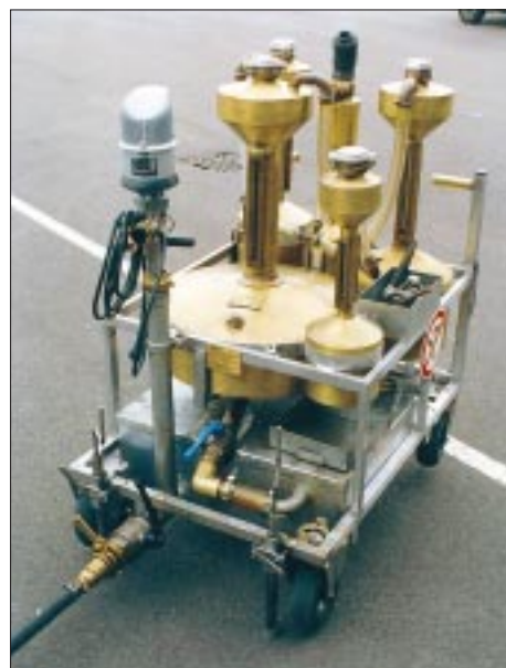
Fig. 4 Wheeled testing facility with storage tank container underneath the provers. The pump on the left is for emptying the container if discharge by gravity is not possible (see dark hose, bottom left).
