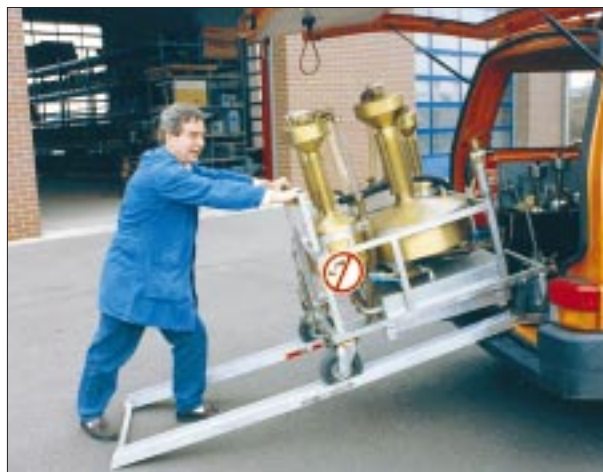
Fig. 3 Testing facility which can be taken out of the vehicle for filling.
