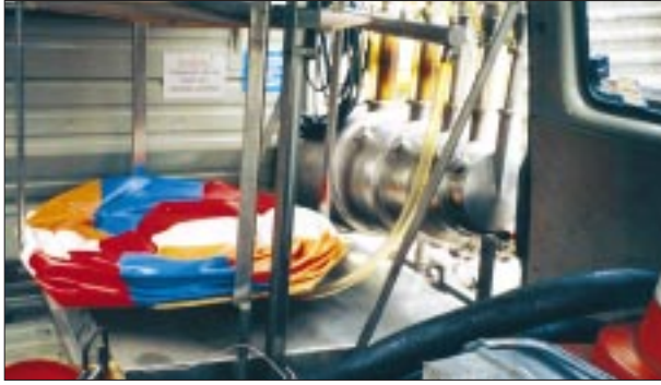
Fig. 8 Testing facility with folded receptacle. When filling the prover, this receptacle collects the escaping gas and air.
