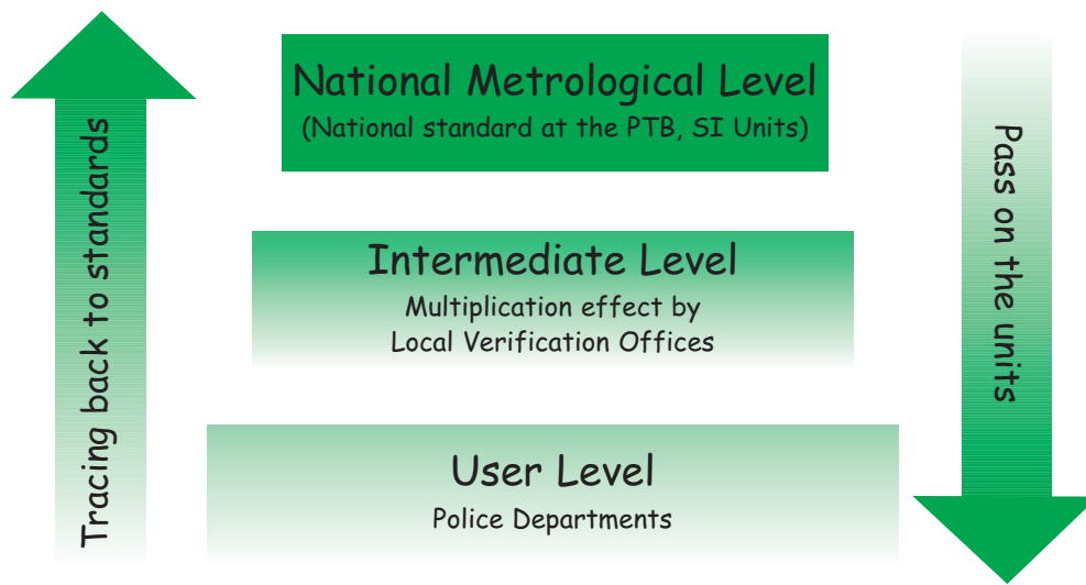
Figure 1 Principle of traceability of breath-alcohol measurements in Germany
