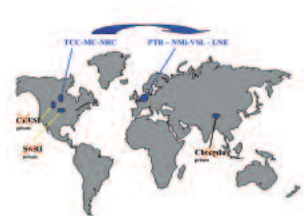
Figure 6 Overview of all high pressure calibration facilities for natural gas worldwide. The facilities in Europe (PTB, NMI-VSL and LNE) are national standards as well the Canadian facility TCC, which is under the supervision of the NRC. All other facilities are private institutes or companies which disseminate their own individual units for gas flow, which are not supervised by a national metrology institute.
