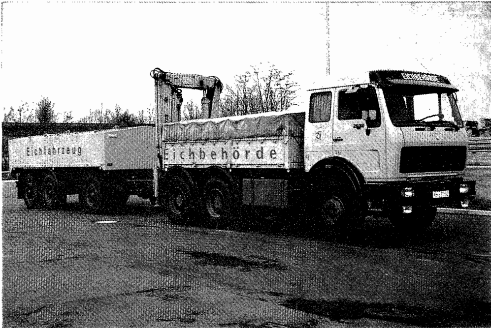
Fig. 1 — Mobile equipment for testing and verification of weighbridges
