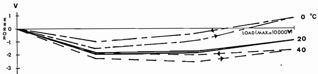
Figure 9 — Performance of a load cell after modification
