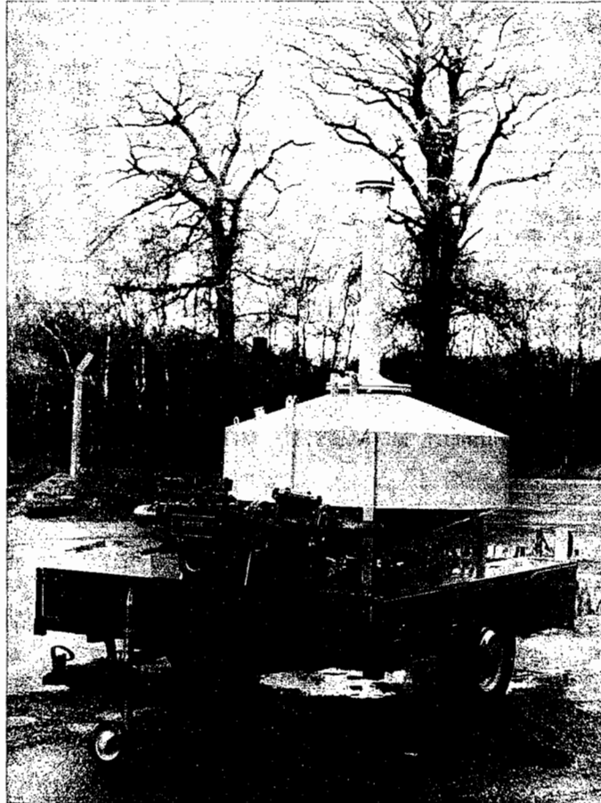
Fig. 19 — EXAMPLE OF A « COMBINATION CALIBRATOR » — A REFERENCE METER COUPLED TO A VOLUMETRIC TANK. (Photo by courtesy of Moore, Barrett & Redwood Ltd.)
